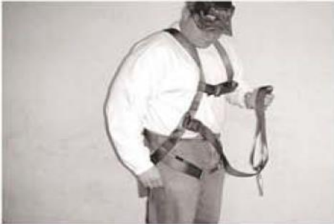
Figure 5- Secure the Linemen's Belt to the Loop on One Side injury or death.
